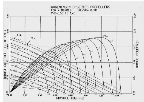
Figure 4. Typical curve of the family of Wageningen propellers. Source: BERNITSAS, M.; RAY, D. y KINLEY, P.  $K_T$ ,  $K_Q$  and efficiency curves for the Wageningen B-series propellers. Department of Naval Architecture and Marine Engineering. University of Michigan.
